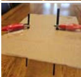
2. Add the carbon rods through the holes in the card, ensuring they do not touch.
