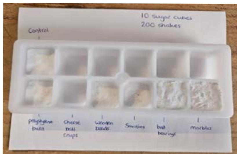
Polystyrene balls and marbles give the largest measurable difference between the amount of ground material produced and how visually coarse/fine the material is.
